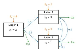
and  $\alpha = 1/2, \beta = 1/24$ . The unit of all the above time is **minute**. Each station has a single queue and unlimited waiting space. The routing probability to other stations and to departure are as shown.
